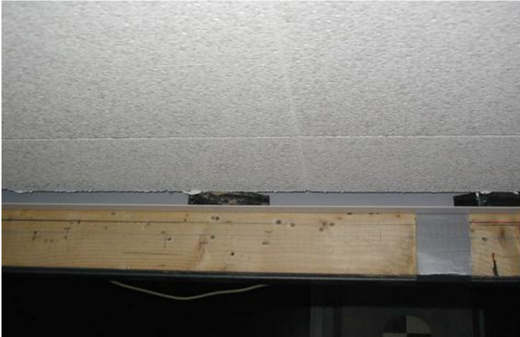
Figure 3-1. Displacement of perimeter tiles over perimeter spring clips following Test 20 for ceiling system CS1.
